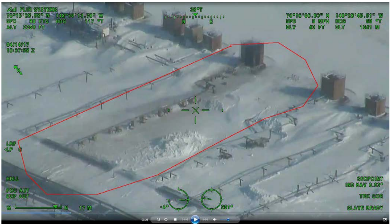
FLIR image from the incident location, taken during an overflight on April 14, 2017. Well 2 and the extent of crude misting is visible on the snow within the red-lined area. [Photo: BPXA]
