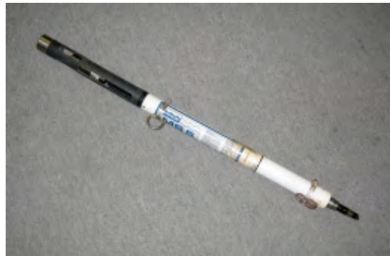
Figure 2: Hydrolab MS-5 minisonde as configured during deployment, sensors are beneath the black guard on left.
