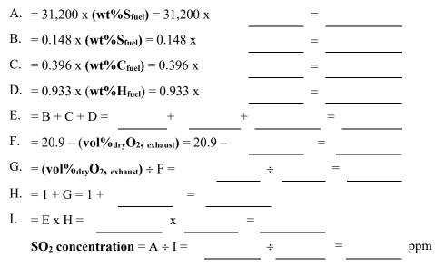
The wt% $S_{fuel}$ , wt% $C_{fuel}$ , and wt% $H_{fuel}$  are equal to the weight percents of sulfur, carbon, and hydrogen, respectively, in the fuel. These percentages should total 100%.
