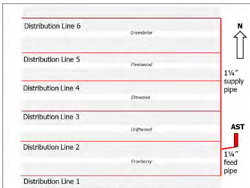
Figure 15. Schematic showing the heating oil distribution network at Four Seasons, based on field evidence. The above ground storage tank (AST) is not to scale.
