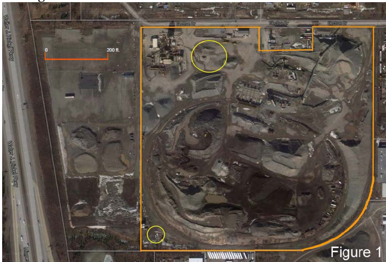
Figure 1: Approximate areas of petroleum hydrocarbon impacts to groundwater circled; areas are located within the northwestern portion and the southwestern corner of the Central Paving site property and occupy an estimated combined total of less than one acre. (Aerial photograph and property boundary from www.anchoragelive.com ).
