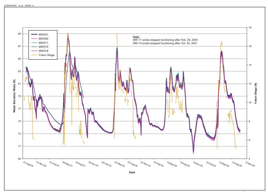
Figure 12-6 Continuous Water Level Monitoring Results Tanana FAA Station, Alaska
