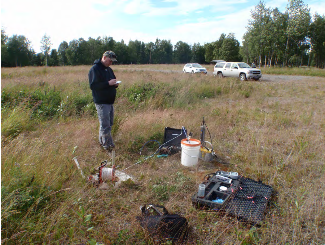
Photo #1: Collecting water samples at Operations Facility MW-3, view NE (8/15/18)
