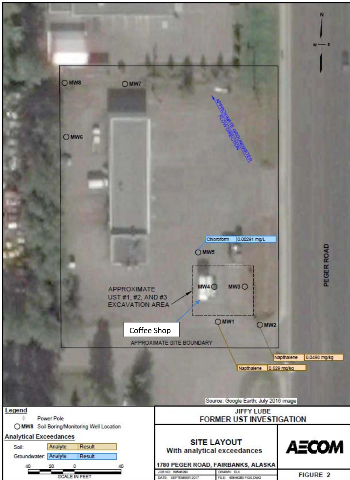
Figure of 2017 Monitoring Well locations and residual contamination in soil and groundwater
