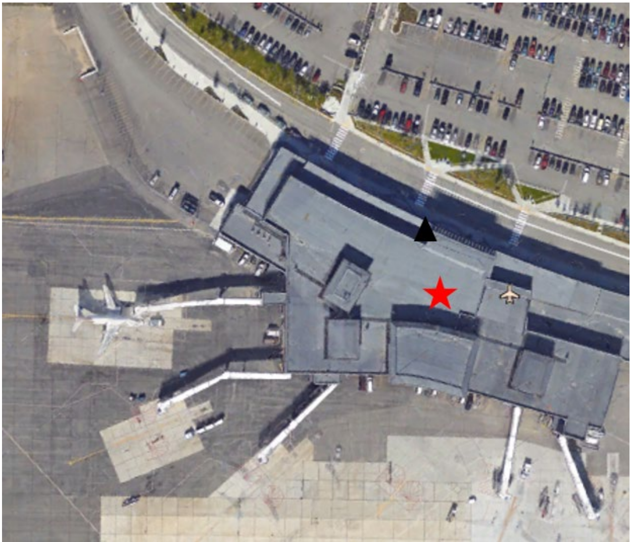
Figure 2. The star indicates the approximate location of remaining soil contamination underneath the new FIA Passenger Terminal. The black triangle indicates the location of the former monitoring well (MW-32) that was sampled in 2007. Image sourced from Google Earth, 2017.
