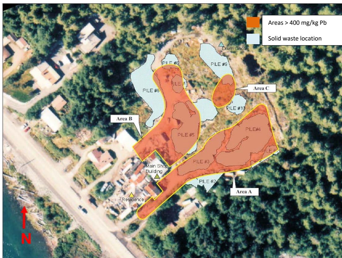
Figure 2: Site Diagram of the Wrangell Junkyard, denoting contaminated areas (Ecology & Environment, June 2002)
