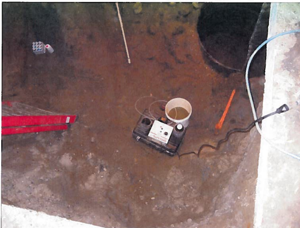
Photo 06 - Groundwater sampling of manually installed temporary sampling point in the bottom of the excavation
