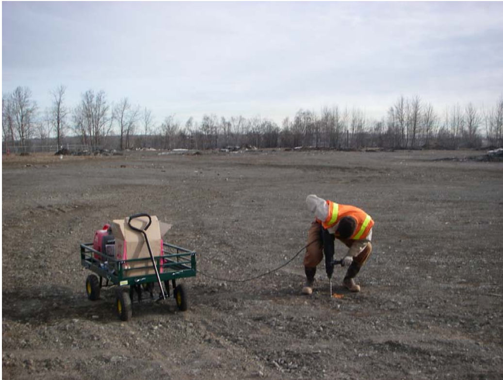
Photograph 5. Drilling passive soil gas monitoring points in April.
