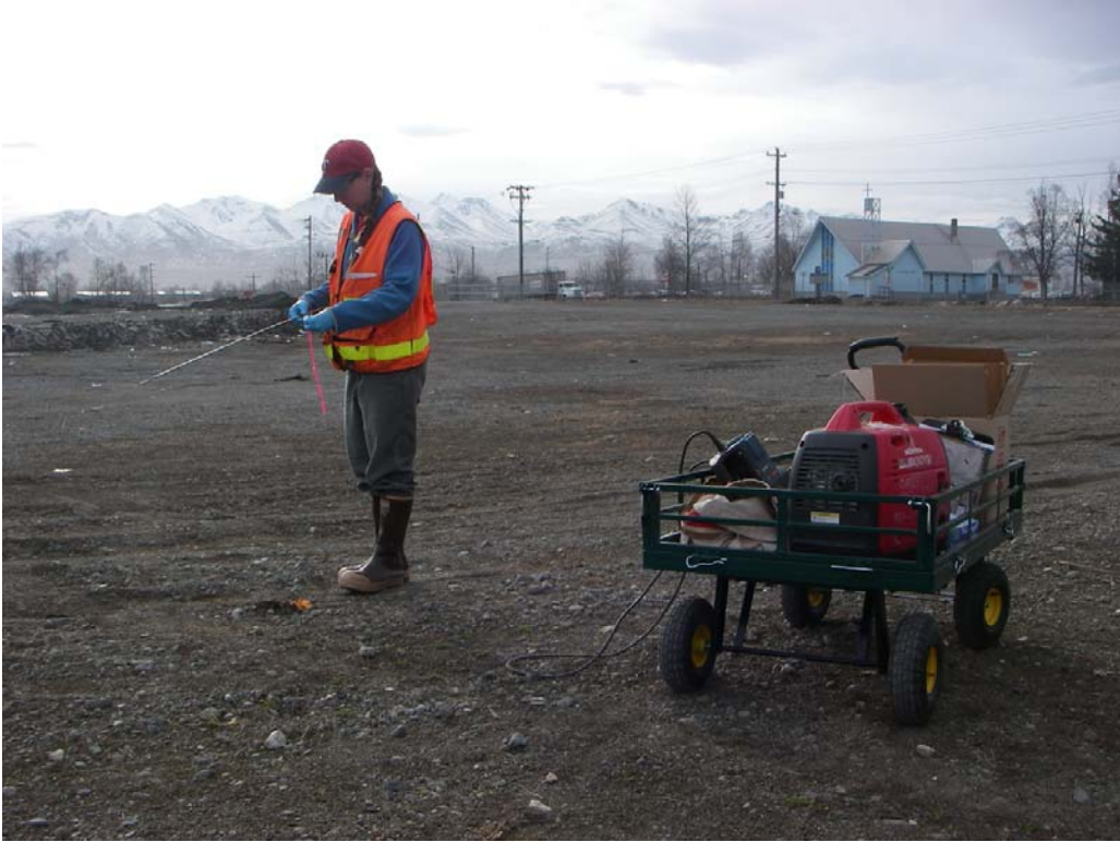
Photograph 7. Preparing to insert passive soil gas sampling module.
