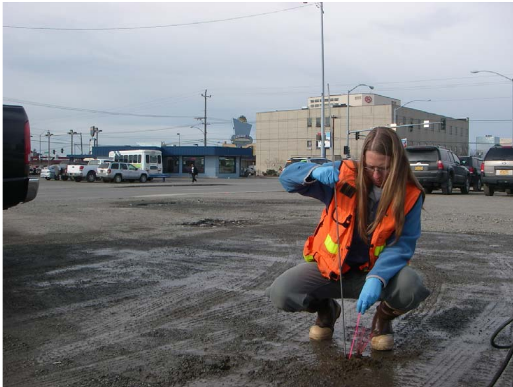
Photograph 9. Inserting passive soil gas sampling module.
