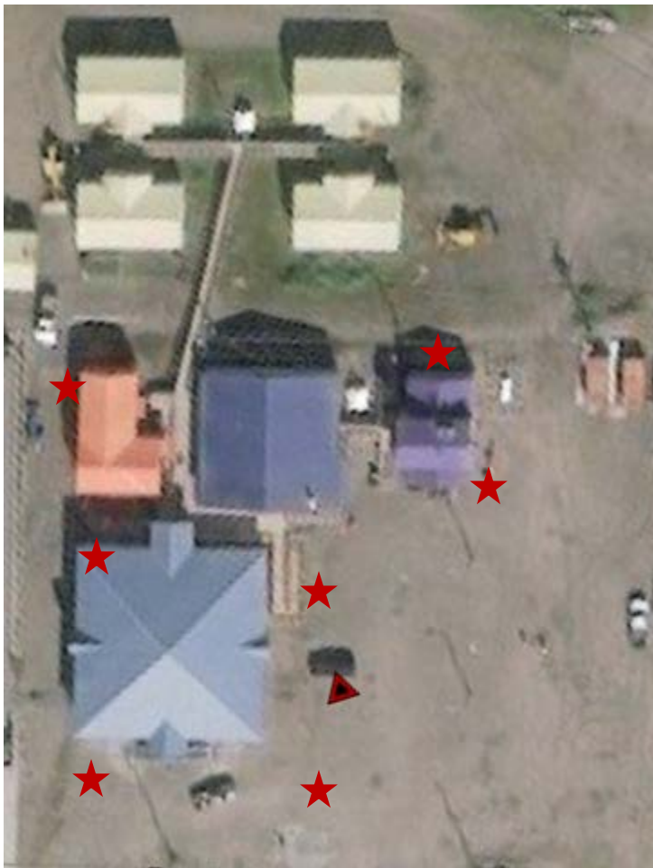
Figure 1. Site figure with stars indicating approximate locations of soil borings where contamination was detected.
