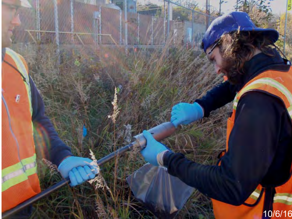
Photo 17. Following removal of surface vegetation with a decontaminated shovel, a coring device and slide hammer were used to collect soil samples at the target depth of 3-4 inches bgs. Bulk soil subsamples for each composite were collected in a Ziploc bag and later homogenized and placed in sample jars for submittal to the laboratory.
