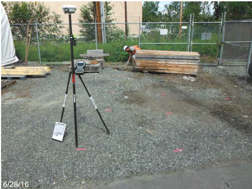
Photo 2. Composite sampling began in the northeast corner of the project area. Samples were collected on a 5' by 5' grid, compositing up to 9 samples. The grid was maintained using a Trimble R8 rover with Virtual Reference Station (VRS) correction service. Sample AP-2 is laid out with pink flags.
