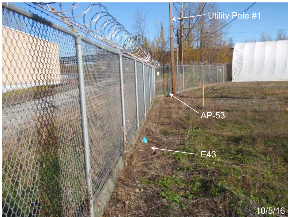
Photo 8. Additional samples were collected along the fence line, including discrete grid locations E43 and composite sample AP-53, shown here. Utility pole #1 is visible adjacent to sample AP-53. The pole is located between samples AP-53 and AP-14, where PCBs were detected at 3.0 mg/kg. Photo faces east.
