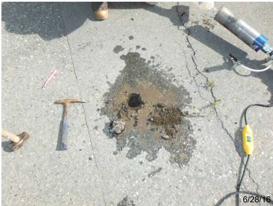
Photo 12. Discrete sample location AP-AA15, collected from the paved area. Soil underneath the pavement was loosened with a decontaminated rock hammer once the pavement core was removed.
