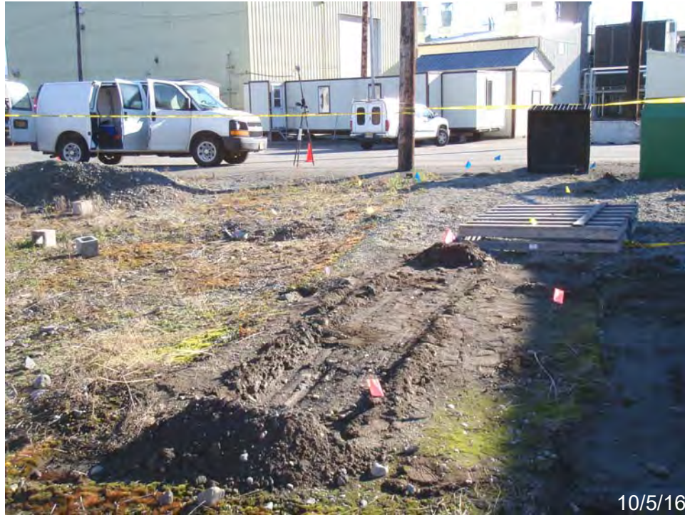
Photo 7. In October 2016, additional surface soil samples were collected in the proposed asphalt paving area to characterize previously un-sampled areas. Samples were collected following removal of the storage container. Collection of soil samples AP-54 through AP-57 is shown. Photo faces south.
