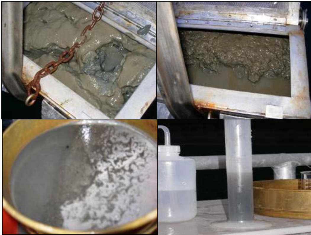
Figure 3-7. Sediment inside of grab, sieving process, and volume displacement method
