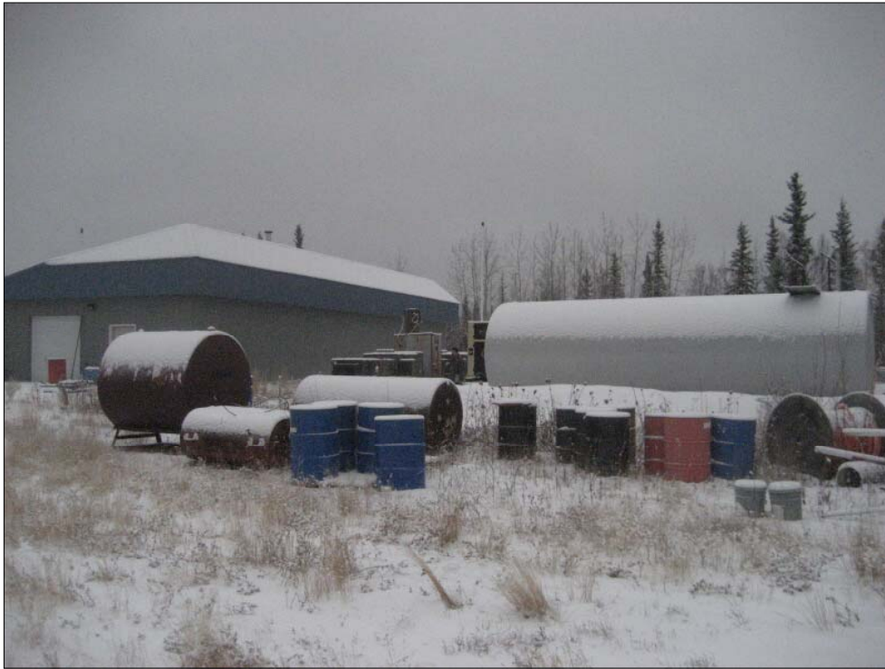
Photo 05 - Tank and drum storage north of 10,000 gallon tank; smaller tanks are empty and drums have been characterized for disposal (new and used antifreeze, lubricating oil, and dielectric oil)
