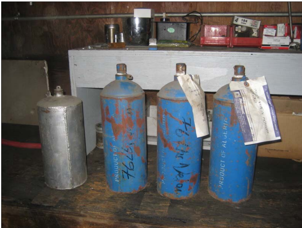
Photo 30 - Steel cylinders (empty) used for transportation/delivery of mercury located inside the Garage/Shop
