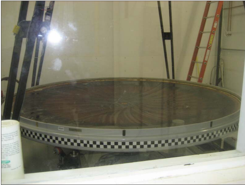
Photo 23 - Rotating mirror in sealed mirror room of LIDAR Building without mercury reflecting surface
