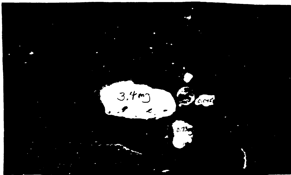
Figure IV-4. Particles of WP isolated from a sample (240) collected in Area C. Counterclockwise from the large particle to the left of the glass bead, the estimated masses are 3.4, 0.73, 0.045 and 0.0049 mg. The glass bead is 0.72 mm in diameter.
