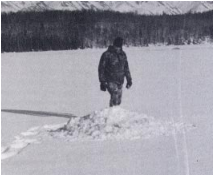
Figure 10. Camouflet formed by a delay-fused 81-mm mortar projectile.
