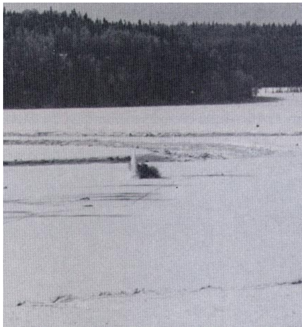
Figure 5. Ricocheting projectile exploding near the ice surface. The white plume of snow and ice shows where the projectile initially hit, and the explosion was just beyond it.
