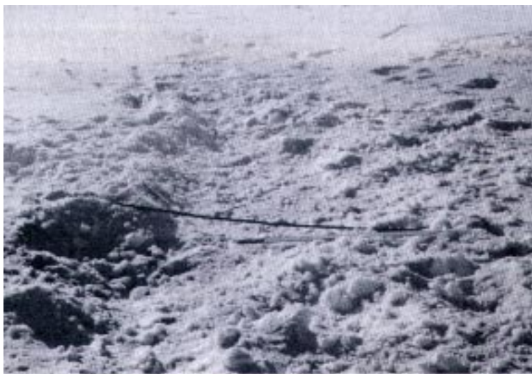
Figure 6. Shallow elongated crater produced by a ricocheting delay-fused projectile.
