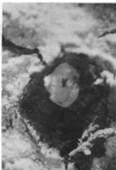
Figure 9. Void in dry sediment formed as P_4 particle sublimed. Dark-colored hygroscopic oxidation products are visible in the sediment surrounding the void.
