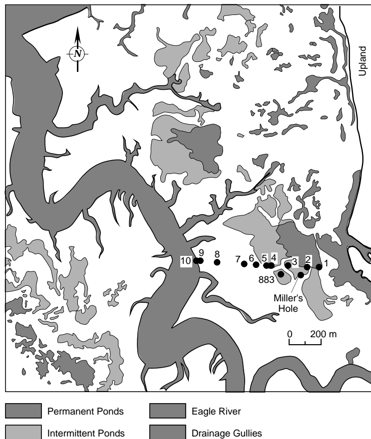
Figure 16. Locations of study sites in Area C. Sediment temperature and moisture were monitored and white phosphorus particles incubated between May and August at sites numbered 1 to 10. Sites 883 and Miller's Hole are field-contaminated sites which were sampled to determine P_4 concentrations.
