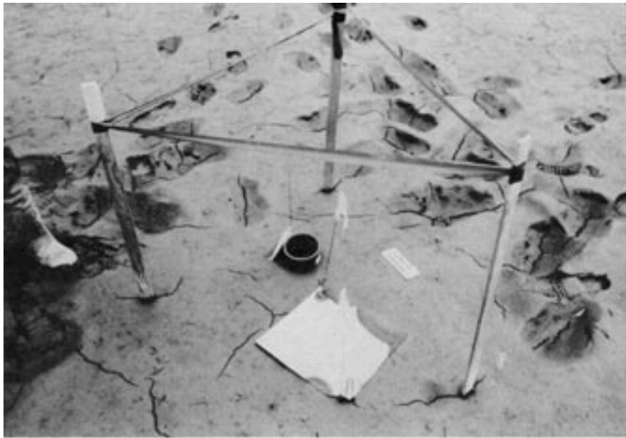
Figure 12. Example of sedimentation station at intermittent pond location showing layout of cup and plate sampler.
