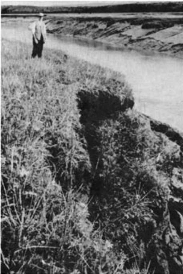
Figure 54. Rotational slump block failure at River Section-North.
