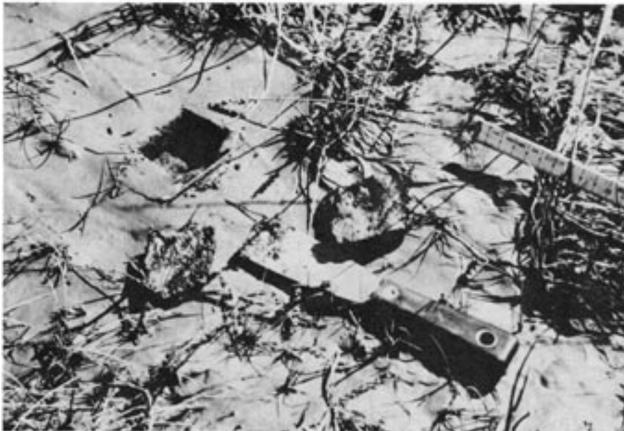
Figure 9. Paint layer depth within block of sediment is measured to define sedimentation rates.
