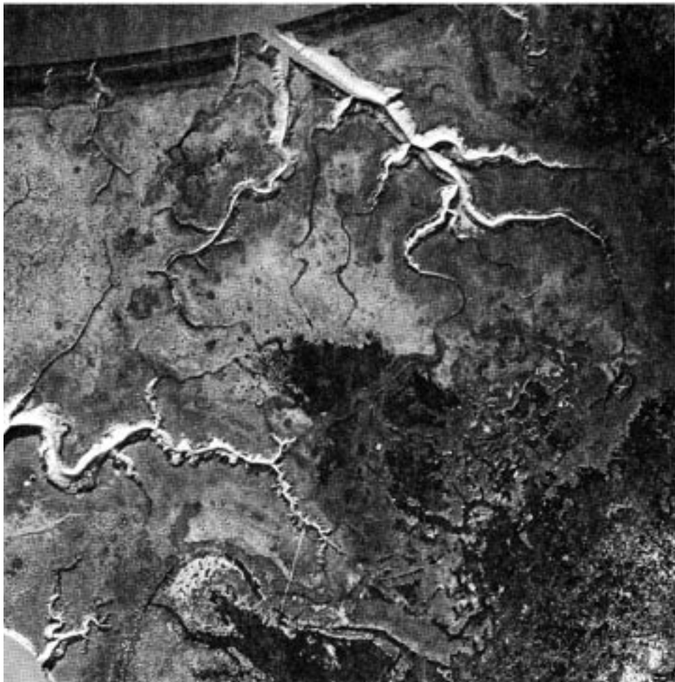
a. Typical active gully erosion following courses of relief drainageways.
