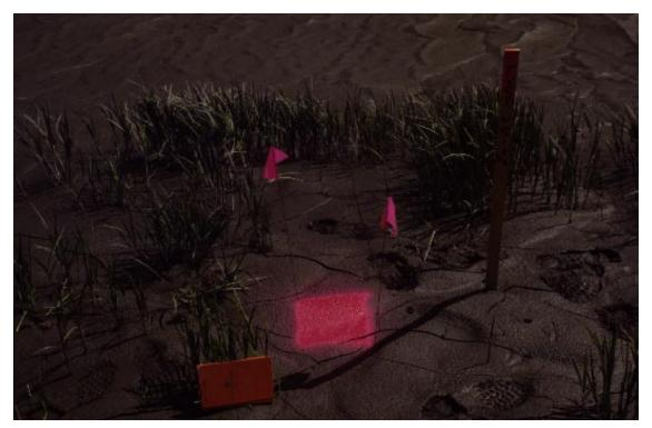
b. Wire flags mark an area of painted ground. Figure 10. Sedimentation measurement techniques.
