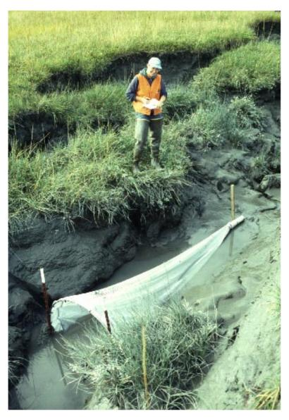
Figure 20. Plankton net used for collecting WP in water transport.
