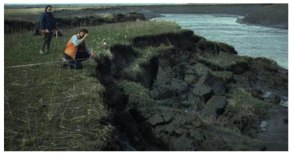
b. Rotational slump blocks visible to right of scarp. Figure 24. Measurements of bank erosion along Eagle River at the River-North site.
