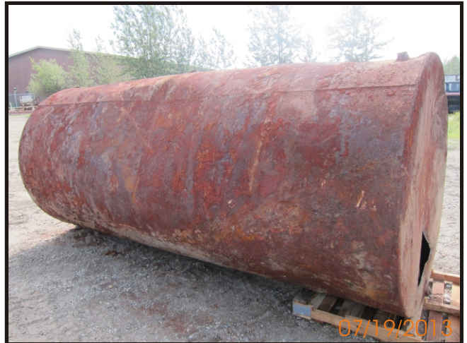
Photograph 6: UST following removal
