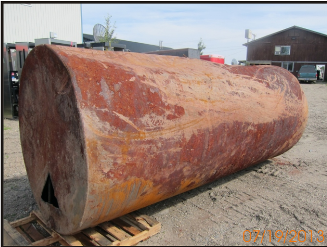
Photograph 5: UST following removal
