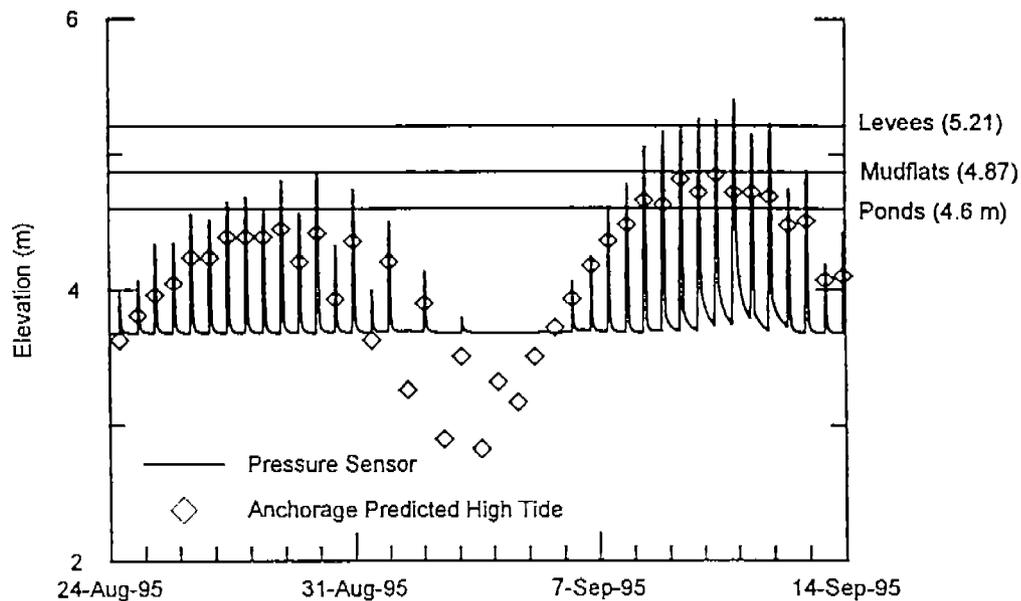
Figure II-1-38. Water elevation record showing elevations required to flood selected landforms and tidal amplification above predicted high tide at Anchorage.
