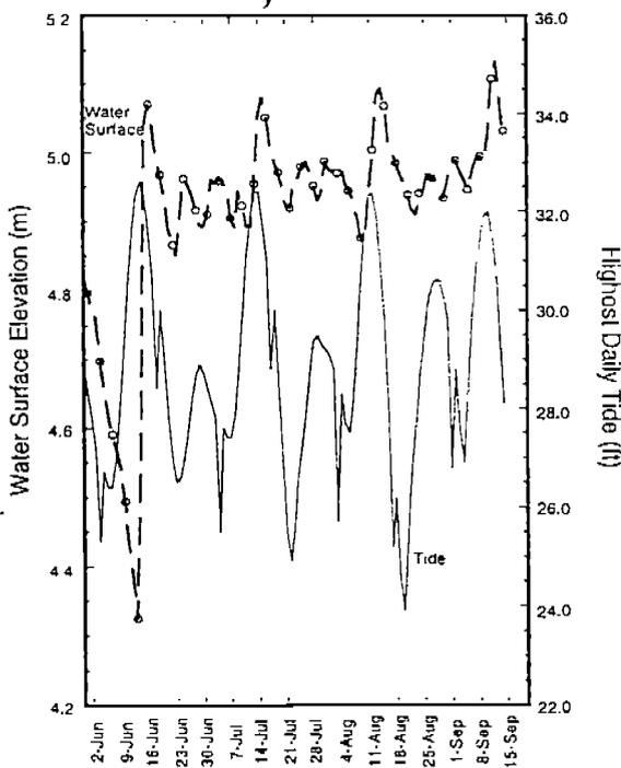
Figure IV-4-8. Water surface elevation at mudflat site and predicted high tides (for Anchorage).
