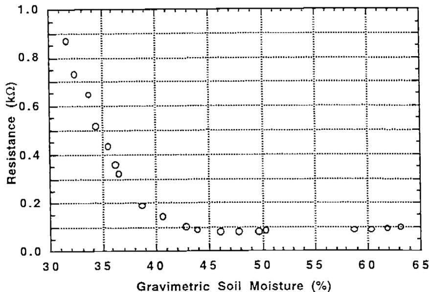
Figure IV-5-5. Soil resistance versus soil gravimetric moisture content of a typical intermittently flooded pond bottom sediment.
