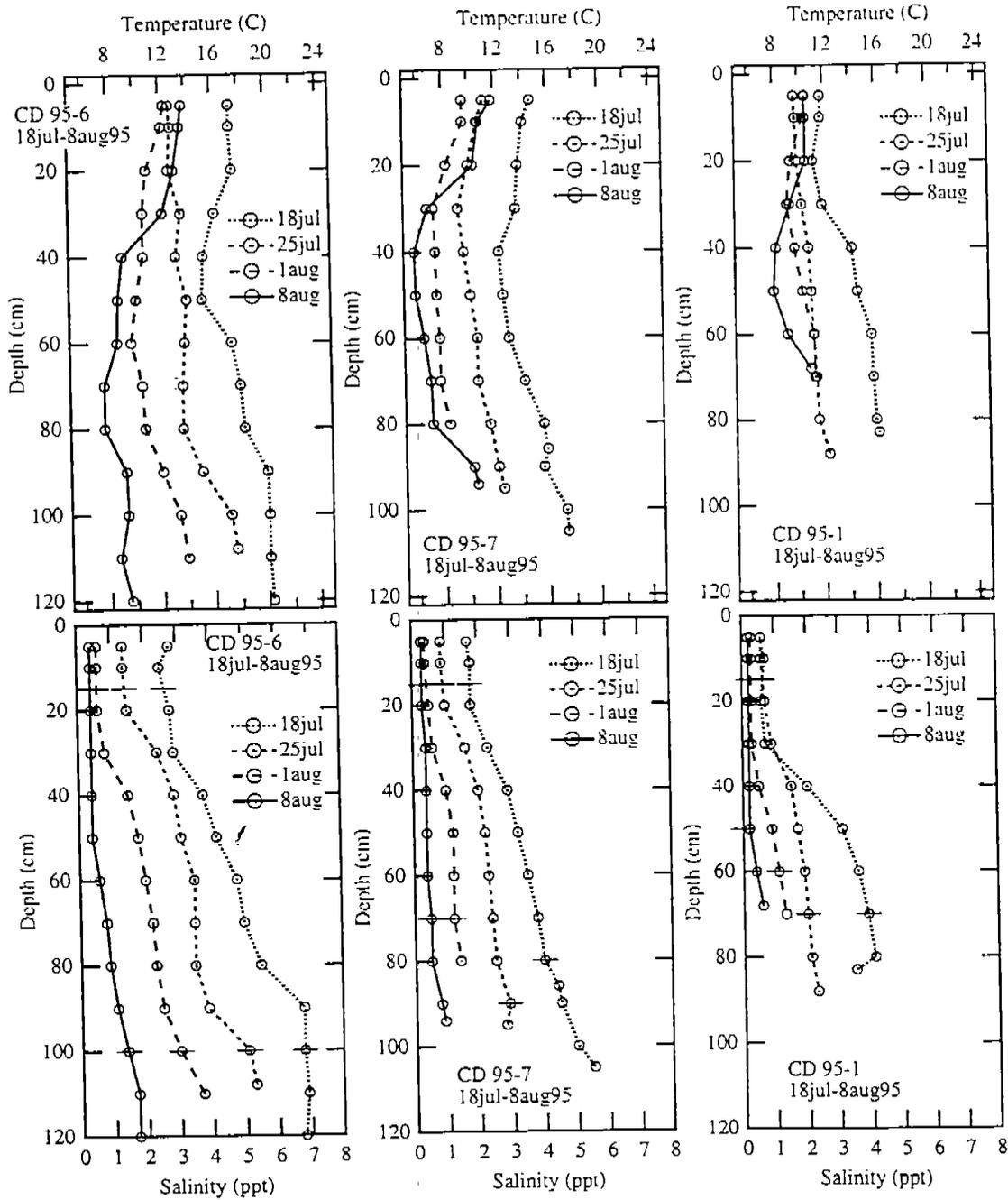
Figure IV-5-9. Salinity and water temperature profiles on the shore transect sampling sites in tide cycle 2, July–August 1995.
