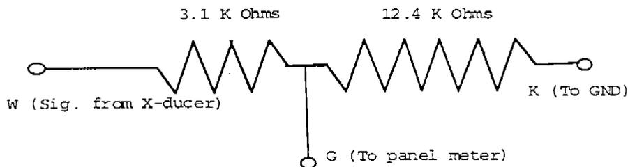
Figure IV-6-6. Sensor voltage divider (Typ. each sensor).
