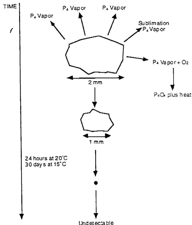
Figure IV-4-14. Conceptual model of the decay of a WP particle in unsaturated sediment.
