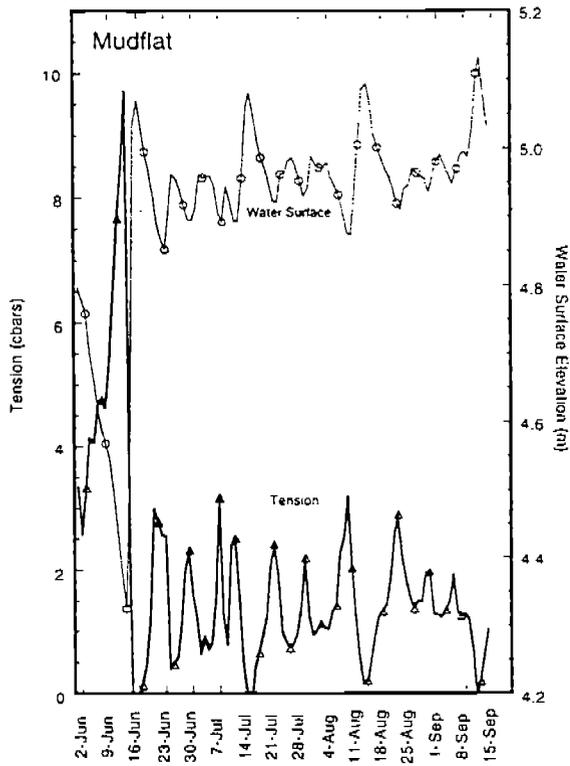
Figure IV-4-6. Water surface elevations and sediment tension (24-hr averages) at the mudflat site.
