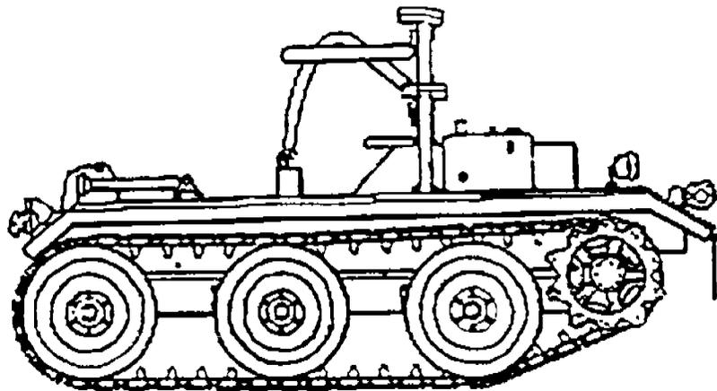
Figure IV-7-7. M501E3 without missile loader.
