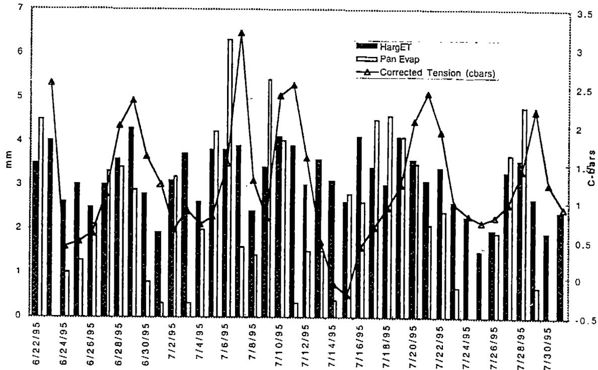
Figure II-2-8. Soil moisture tension, evapotranspiration and pan evaporation.
