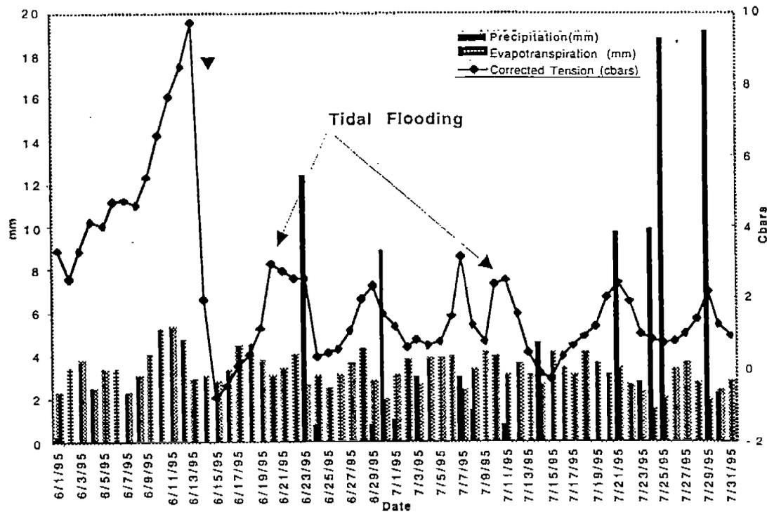
Figure II-2-9. Soil moisture tension, precipitation and calculated evapotranspiration, June–July 1995, Eagle River Flats.
