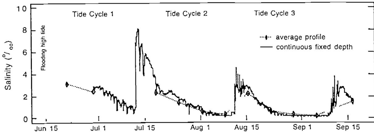
Figure IV-5-14. Comparison of the continuous salinity at a fixed depth and average salinity in the profile at CD-1 in 1995.
