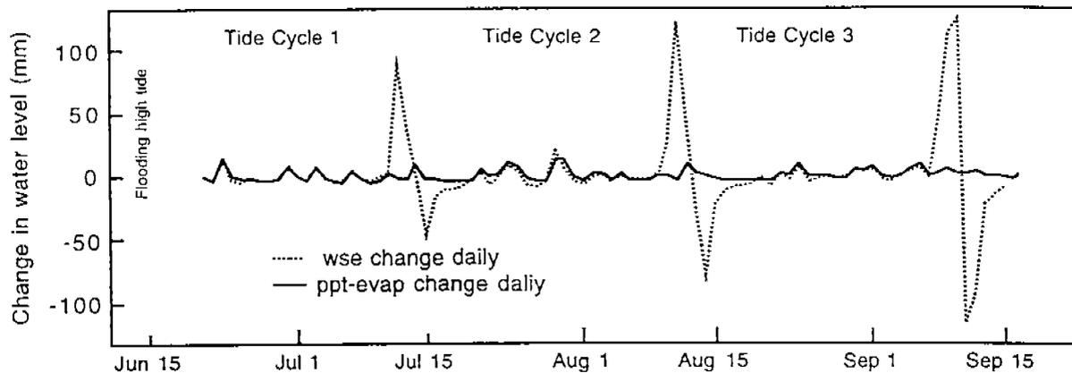
Figure IV-5-19. Comparison of changes in the pond water surface elevation and daily evaporation and precipitation in 1995.
