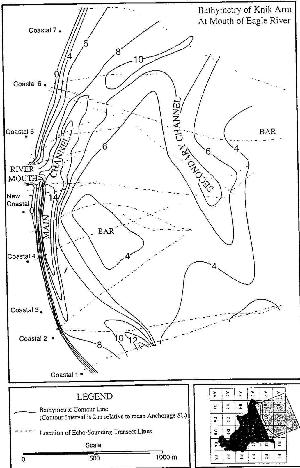
Figure II-1-53. Bathymetry of Knik Arm near mouth of the Eagle River and adjacent to the coast of ERF.
