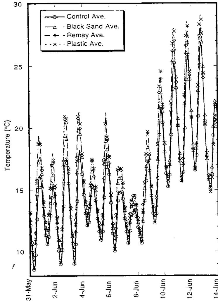
Figure IV-4-11. Diurnal temperature (average of four replicates) variations in sediment (5-cm depth) under control (bare) and three treatments during first two weeks of June.
