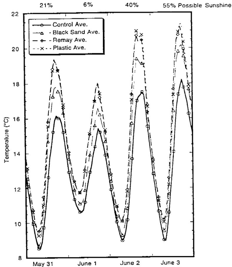
Figure IV-4-12. Diurnal temperature (average of four replicates) variations in sediment (5-cm depth) under control (bare) and three treatments May 31 to June 3 and percent possible sunshine.
