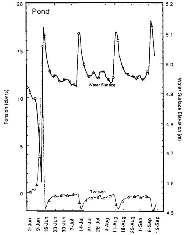
Figure IV-4-7. Water surface elevations and sediment tension (24-hr averages) measured at the pond site.
