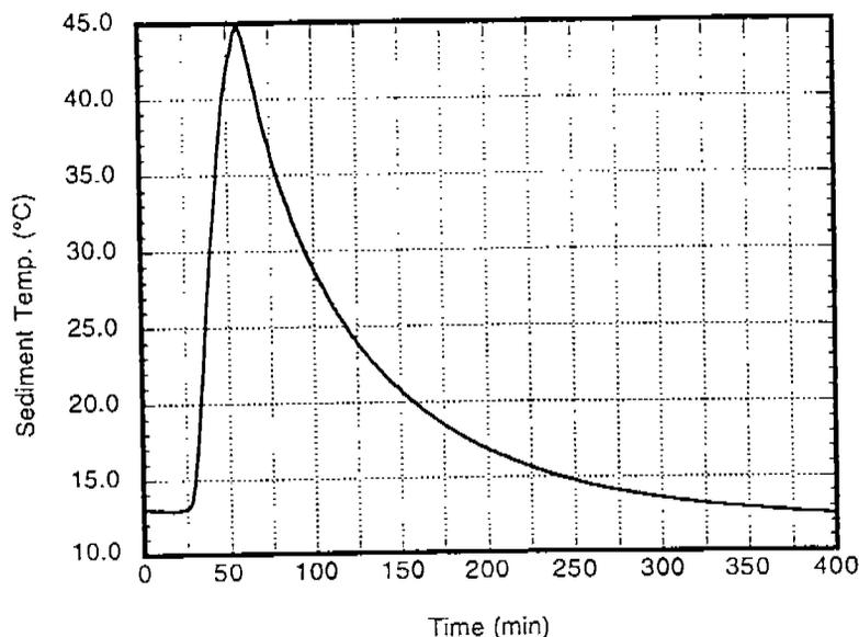
Figure IV-4-15. Temperatures in sediments equilibrated in a cool environmental chamber, and briefly warmed with a heat gun. Heat source was applied at 25 min and removed at 55 min. WP particles were recovered 24 hr after the heating event.
