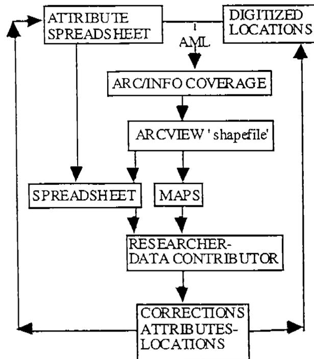
Figure V-1-7. Error checking procedure for ERF database.
