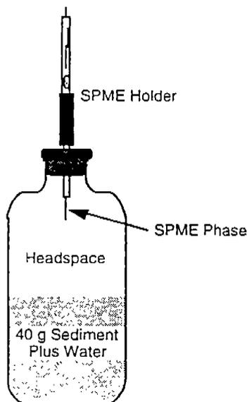
*Figure IV-3-3. Solid phase micro-extraction (SPME) of a sediment sample to test for the presence of WP. Following exposure to the headspace above a sample, the SPME phase is transferred directly to the injection port of the gas chromatograph.*
