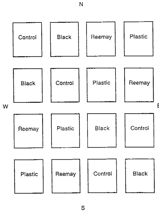
Figure IV-4-2. Arrangement of 1-m<sup>2</sup> plots. Control = Bare, Black = Black Sand, Reemay = spun-bonded polyester fabric, Plastic = Fast Start (porous polyethylene).
