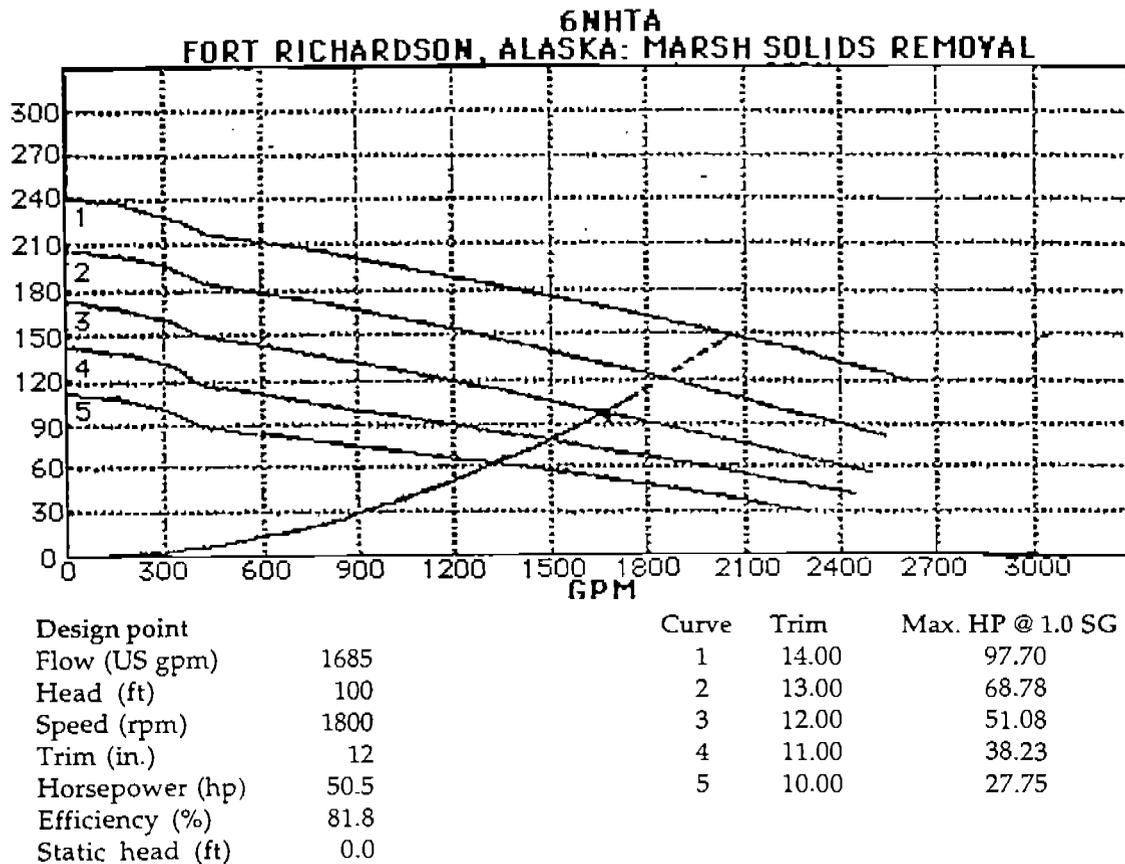
Figure IV-6-7. Pump curves for 1800-rpm impeller. (Adapted from Cornell 1995.)
