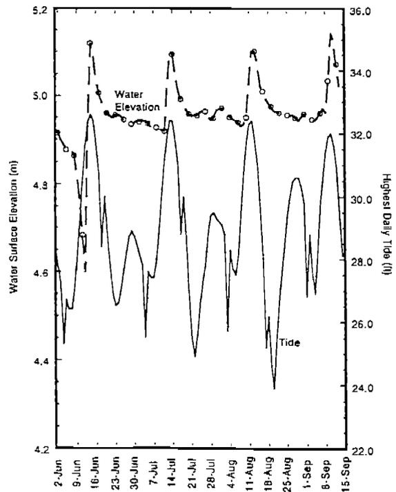
Figure IV-4-9. Water surface elevation at the pond site and predicted high tides (for Anchorage).
