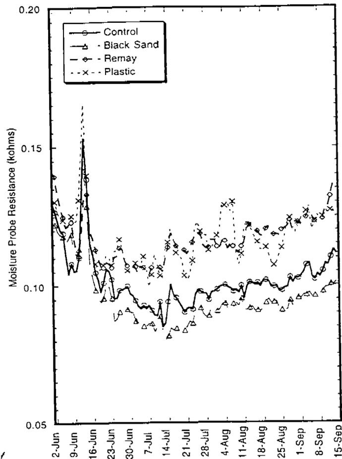
Figure IV-4-13. Moisture probes resistances at 5-cm depth for control (bare) and three treatments at mudflat site. A rise in resistance indicates that the sediments are drying.
