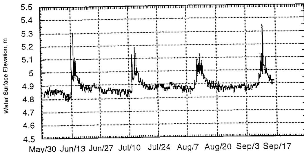
Figure IV-5-6. Water surface elevation for the Bread Truck pond from 31 May to 15 September.
