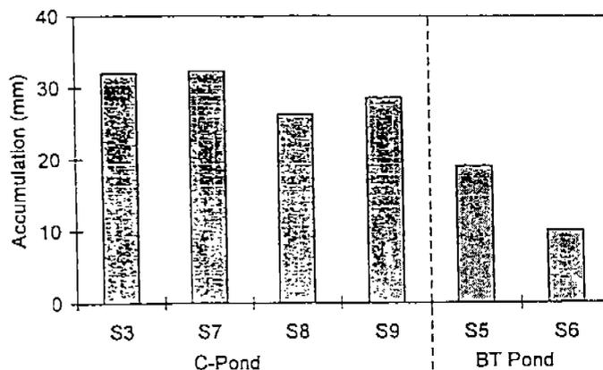
Figure II-1-51. Fall 1995 measurements of accumulation at sedimentation stations established in 1992.
