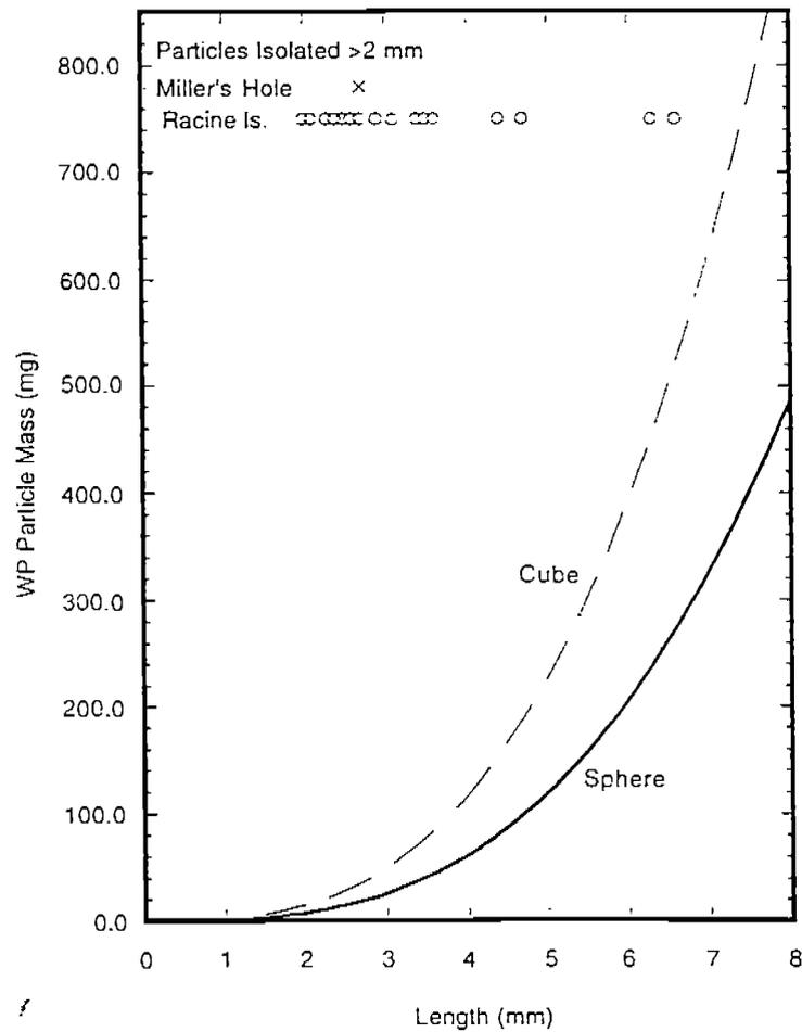
Figure IV-3-9. Mass of cubic or spherical WP particles corresponding to the range of the lengths of particles measured in samples in ERF.
