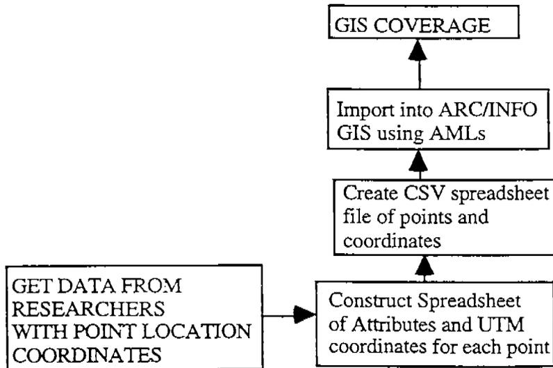
Figure V-1-6. Flow of data from researchers into the ERF GIS database beginning with researcher-supplied locational data.
