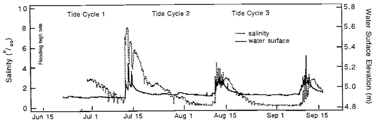
Figure IV-5-15. Water surface elevation and salinity at CD-1 in 1995.
