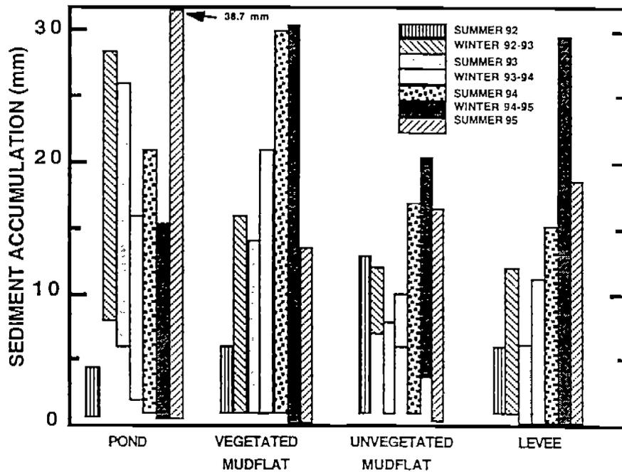
Figure II-1-46. Variations in sedimentation rate as a function of landform type.
