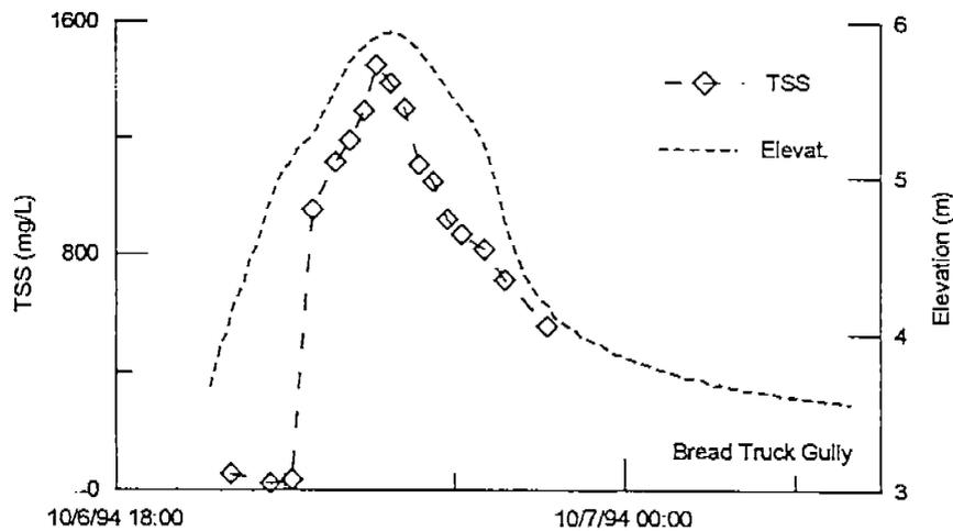
Figure II-1-44. Typical TSS variation through a flooding tide.
