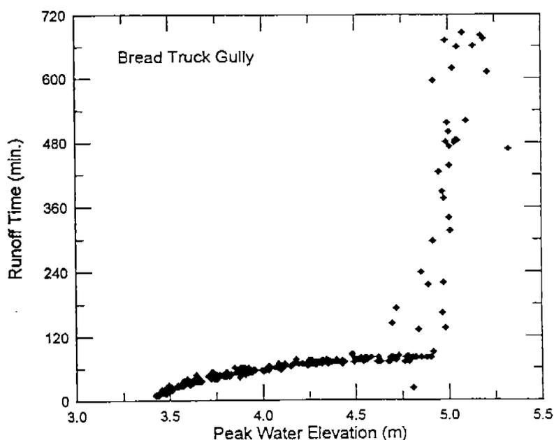
Figure II-1-41. Run-off time versus peak water elevation at Bread Truck Gully. The change in slope reflects the effect of pond drainage where run-off is extended once ponds are flooded.
