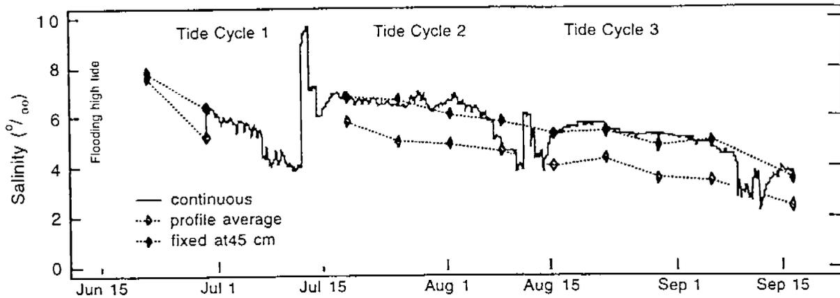
Figure IV-5-17. Comparison of the continuous salinity at a fixed depth, average salinity in the profile and salinity at fixed depth of 45 cm at CD-1 in 1995.
