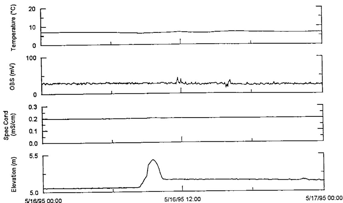
Figure II-1-37. Water quality data from the Eagle River site showing the effect of water damming caused by a flooding tide.
