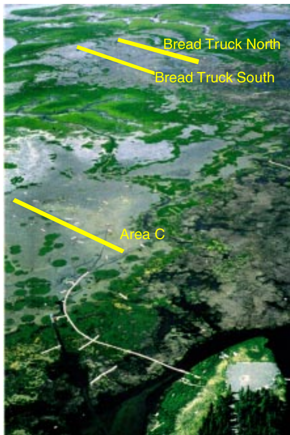
Figure III-2-2. Aerial oblique photo taken in June 1997 showing the main pond of Area C that was drained by pumping and the Bread Truck Pond that was drained by ditching. Transects were established across these ponds, and grid composite samples were collected perpendicular to the transect at 50-m intervals.
