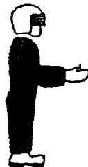
LAND HERE: Extend arms toward landing area with wind at your back.
