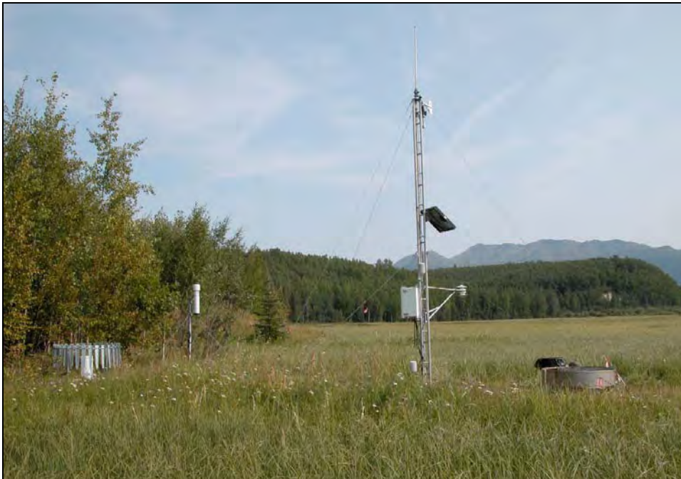
Figure III-3-1. Eagle River Flats meteorological station located along the edge of EOD pad in Area C. Note the 4-m tower in right center, the evaporation pan to the right, and the shielded rain gage to the left.
