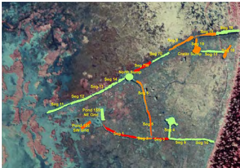
Figure III-2-7. Locations of multi-increment samples collected in C Marsh ditches in 2005. Red and orange indicate white phosphorus was detected. Green indicates that white phosphorus was not detectable in the samples.
