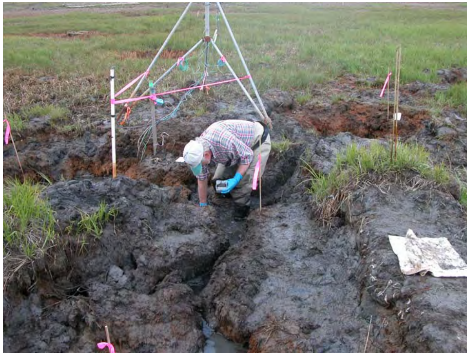
Figure III-2-5. June 2005 sampling of BIP craters in C Marsh. The craters were drained in May 2005 using a small gasoline-powered pump to facilitate remediation and sampling.
