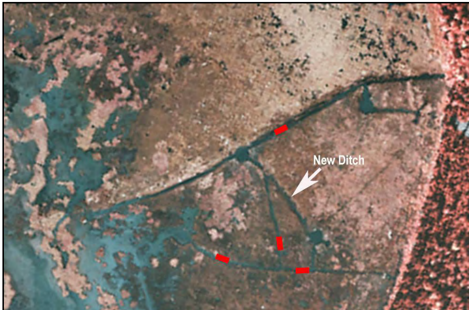
a. Ditch sections (red rectangles, 5-m-long) where particulate WP was detected in 2006.
