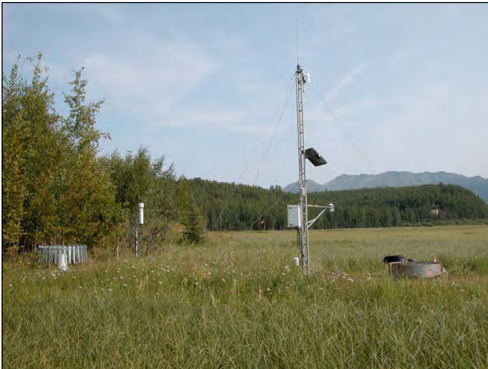
Figure III-3-1. Eagle River Flats meteorological station located along the edge of the OB/OD pad in Area C. The 4-m tower is located in the right center, the 1.22-m-diameter evaporation pan is located to the right, and the shielded rain gage is located to the left.
