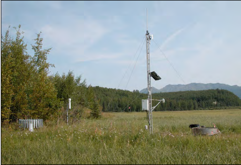
Figure III-3-1. Eagle River Flats meteorological station located along the edge of the OB/OD pad in Area C. The 4-m tower is located in the right center, the 1.22-m-diameter evaporation pan is located to the right, and the shielded rain gage is located to the left.
