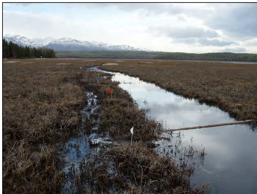
Figure III-2-14. View looking south down the cross ditch. A 70 m long area was subdivided into 5-m long sampling units. White phosphorus was not detected in any sample.
