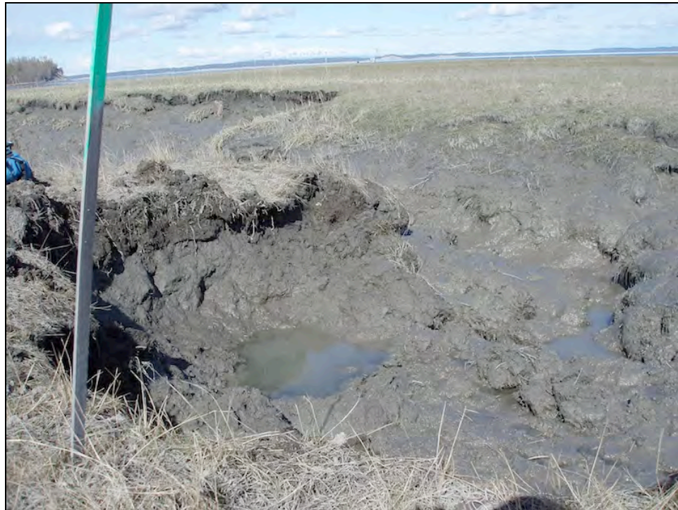
Figure III-2-20. Ground view crater from the detonation of a 4.2-inch WP mortar projectile in a gully in May 2010.
