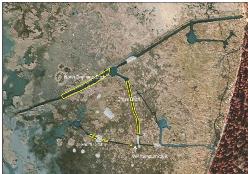
Figure III-2-13. Aerial image showing locations (outlined in yellow) within the drainage ditches that were sampled in 2010. White phosphorus was not detected.
