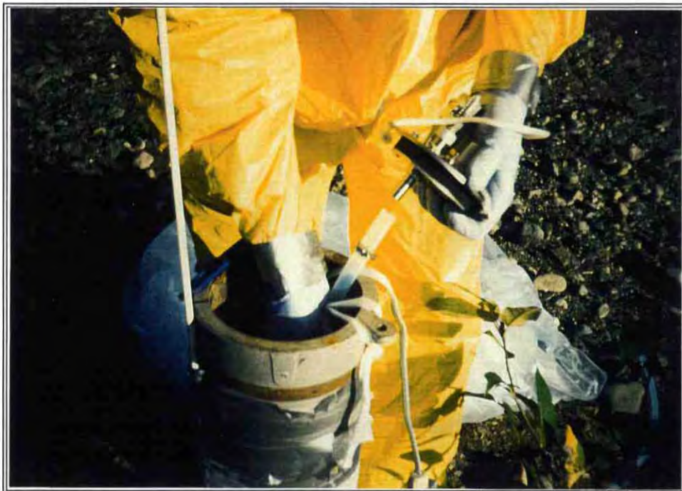
PHOTO 14: The well cap is being attached to the sampling tube.
