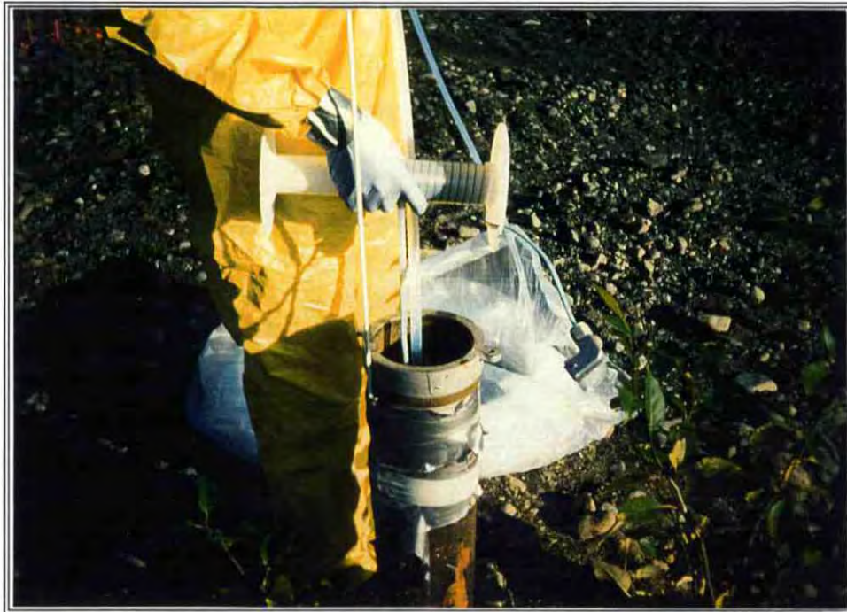
PHOTO 13: A dedicated pump is being lowered into a well. The pump is connected to a power cable and a sampling tube.
