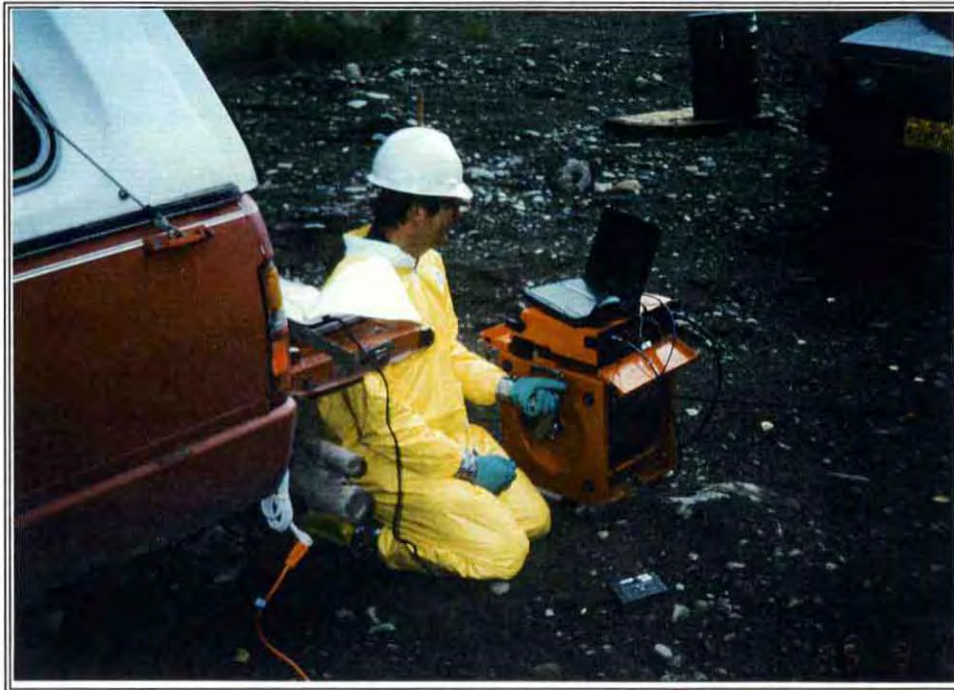
PHOTO 11: The downhole geophysical contractor is lowering an instrument into a well and observing the readings on the computer.
