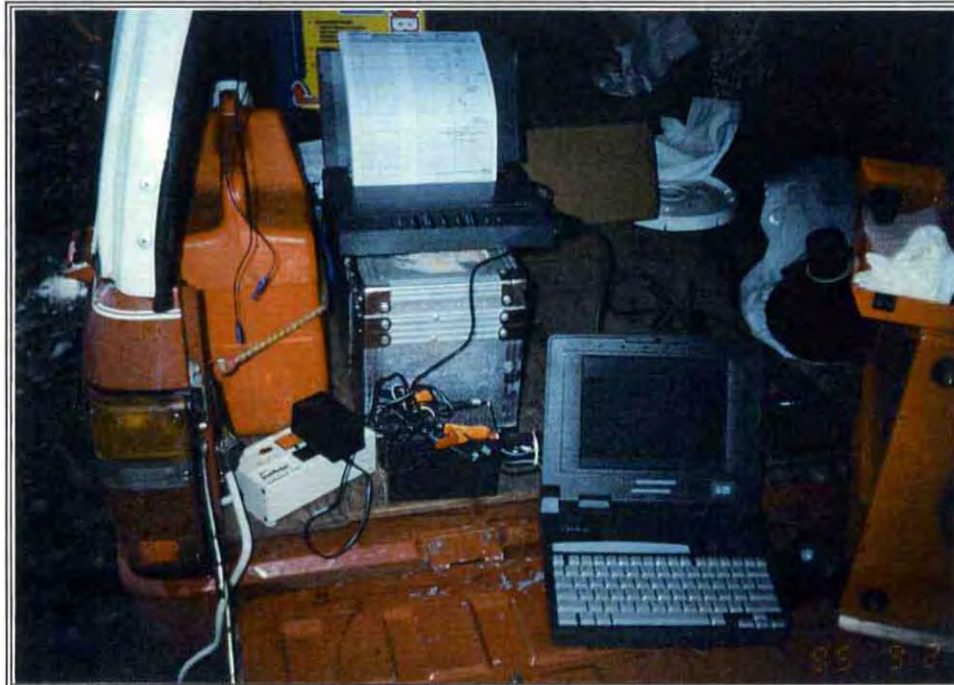
PHOTO 12: Rough drafts of the downhole geophysics logs could be printed out and reviewed in the field.
