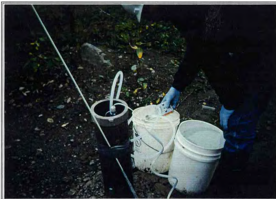
PHOTO 16: Water quality measurements were collected while purging the monitoring wells. The wells were sampled when the water quality parameters stabilized.
