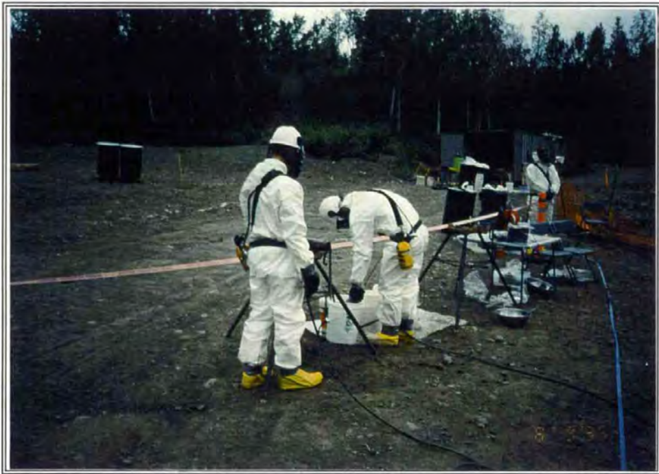
PHOTO 4: The split-spoon is being cleaned and reassembled. EOD specialist is standing by in background.
