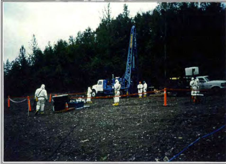
PHOTO 1: Preparing to drill soil boring in Area A-4. Field personnel are wearing Level B PPE.
