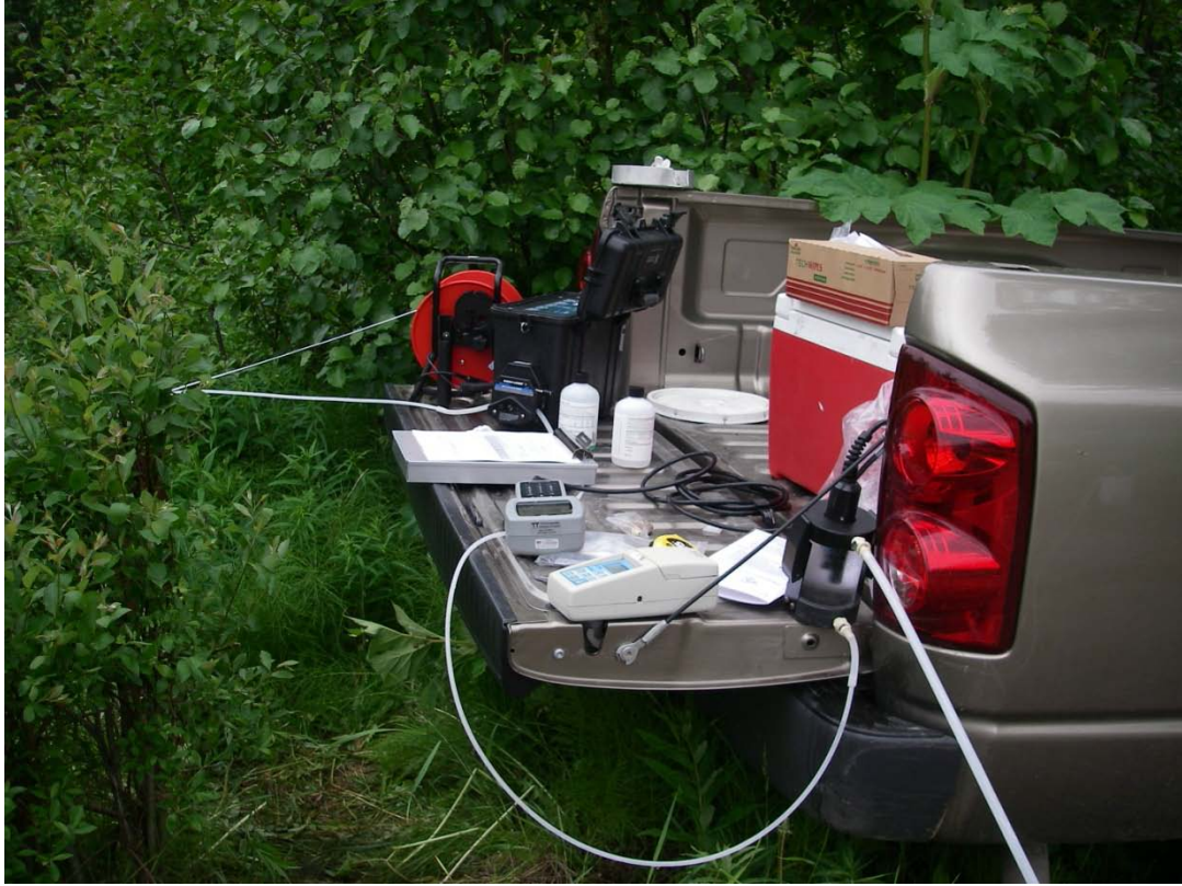
Photo 11: AP-3503, looking SE, peristaltic pump setup
