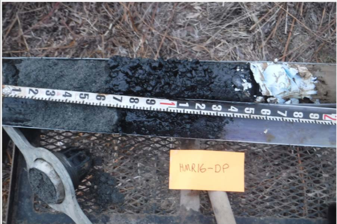
Photo 4: Core from test boring HMR16-DP showing discolored soil with a petroleum odor directly below the foam board in the middle of the core. 2/18/2016
