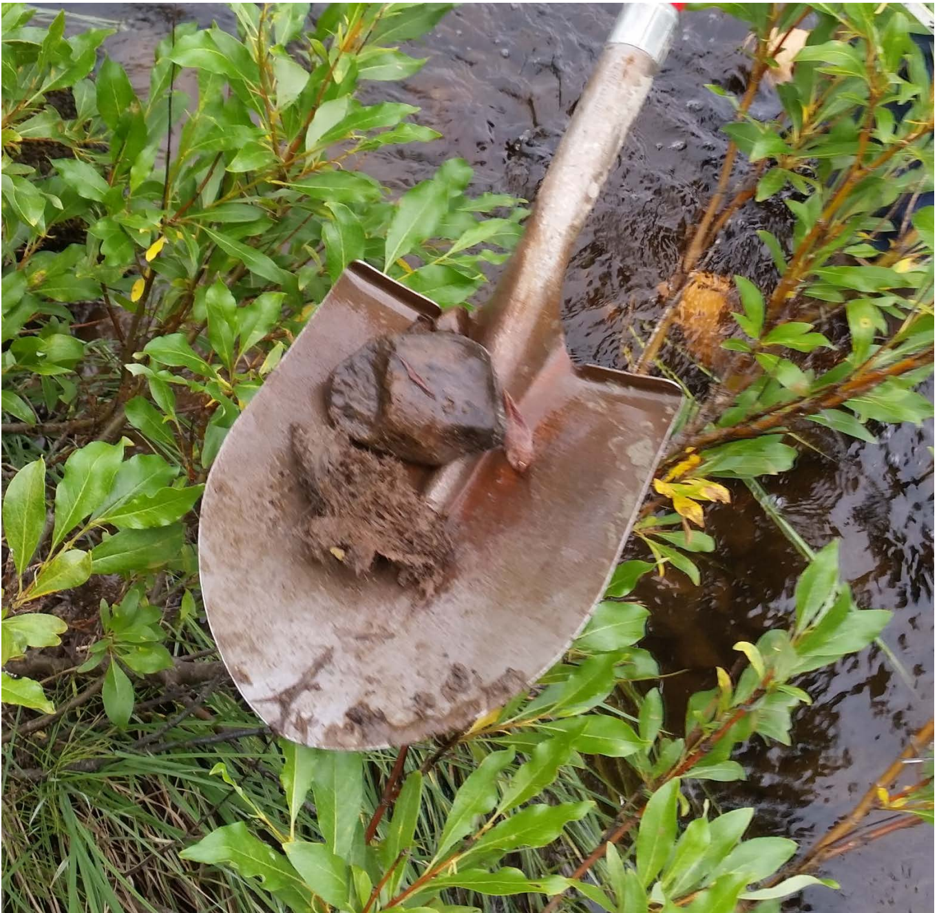
Photo 2: Inspection of stream bank sediments during shovel sheen testing. A survey tape (upper right) was used to measure out testing locations.
