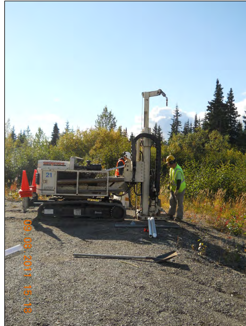
Typical Direct-Push Drilling Methods
