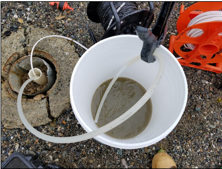
Purge water from RSE-3.
