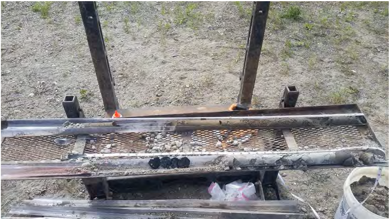
Photo 11: Boring BH1 0 to 4 foot (ft) soil core with FTP liner components visible at approximately 1.5 ft below ground surface (June 7, 2018).
