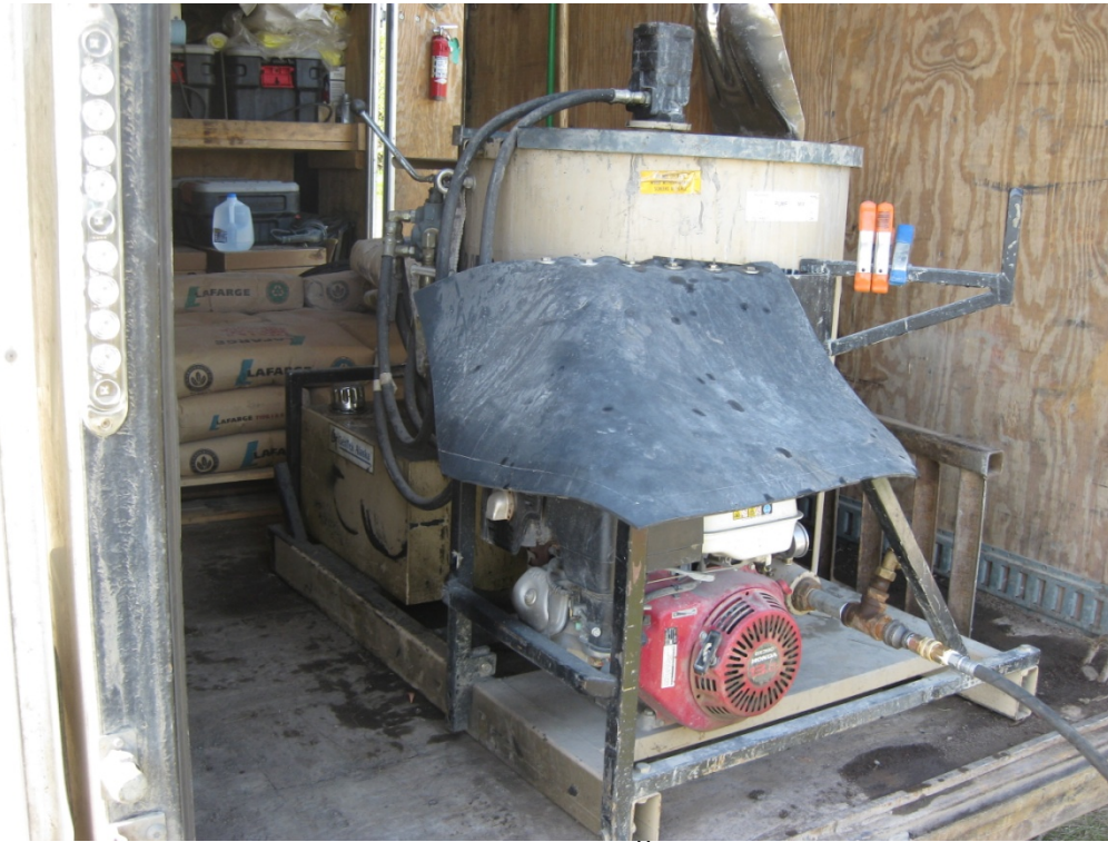
Figure 2.3 Grout Pump Used to Mix EHC ® and Hematite Powder Slurries
