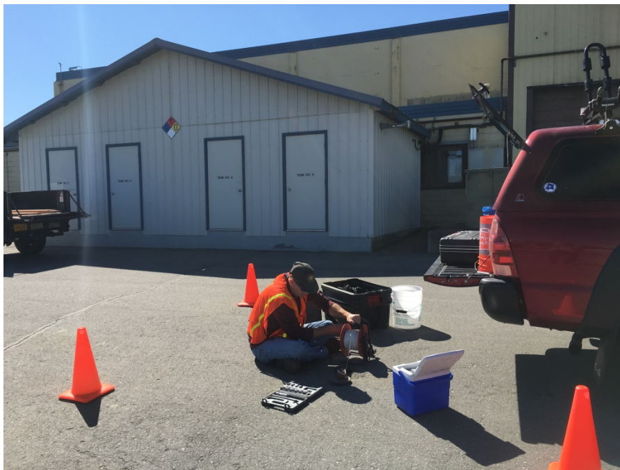
Photo 4: Monitoring Well MW-7, measuring the water level. Location is north of Transformer Shop.
