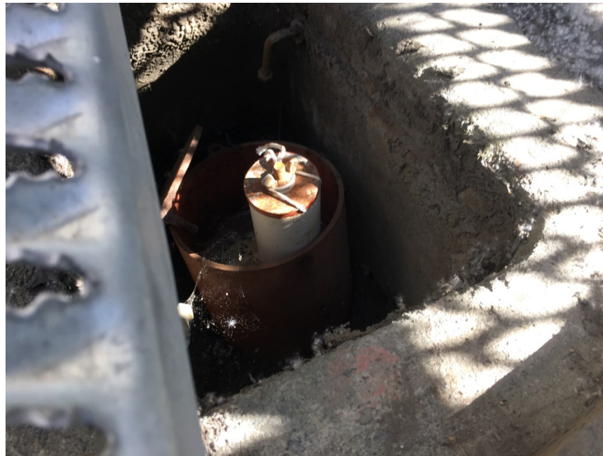
Photo 2: Monitoring Well MW-5 located in a cement utility enclosure under staircase.
