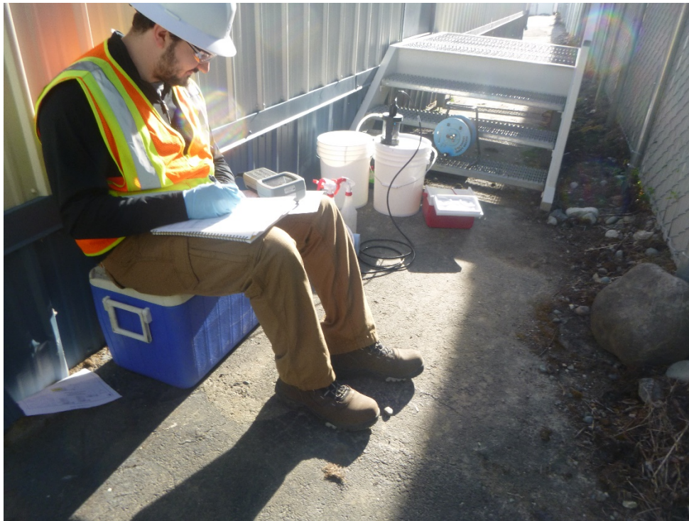
Photo 1: Monitoring Well MW-5 TS, located under the stairs, being purged prior to sampling.
