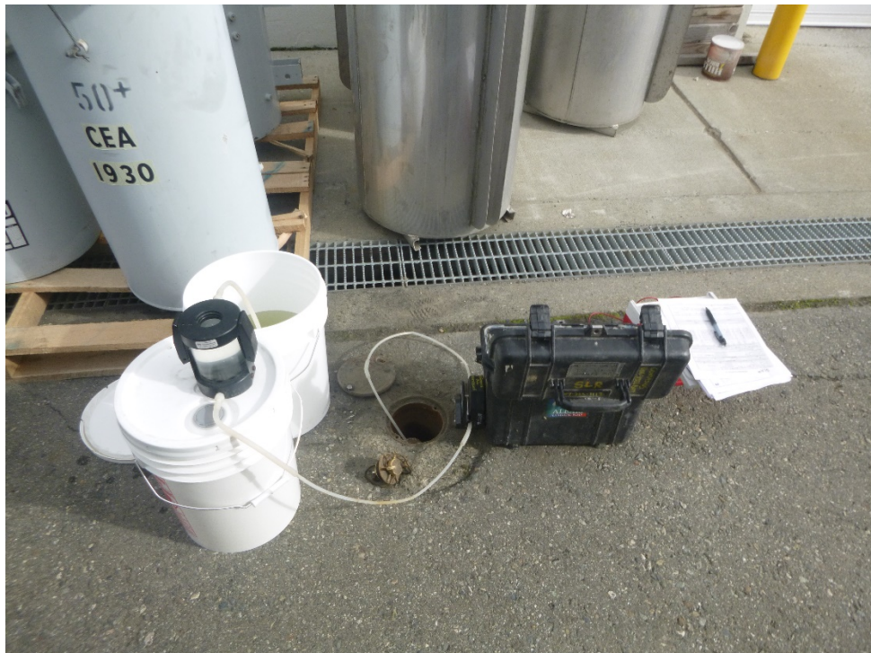
Photo 2: Monitoring Well MW-9 TS as it was being purged on 7/30/18. The well was not sampled until 8/3/18, after being purged dry on 7/31/18. The well is located south of the Transformer Shop.
