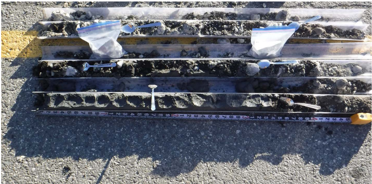
Figure 1. Typical soil conditions showing granular fill soil over fine-grained tidal silt deposits.
