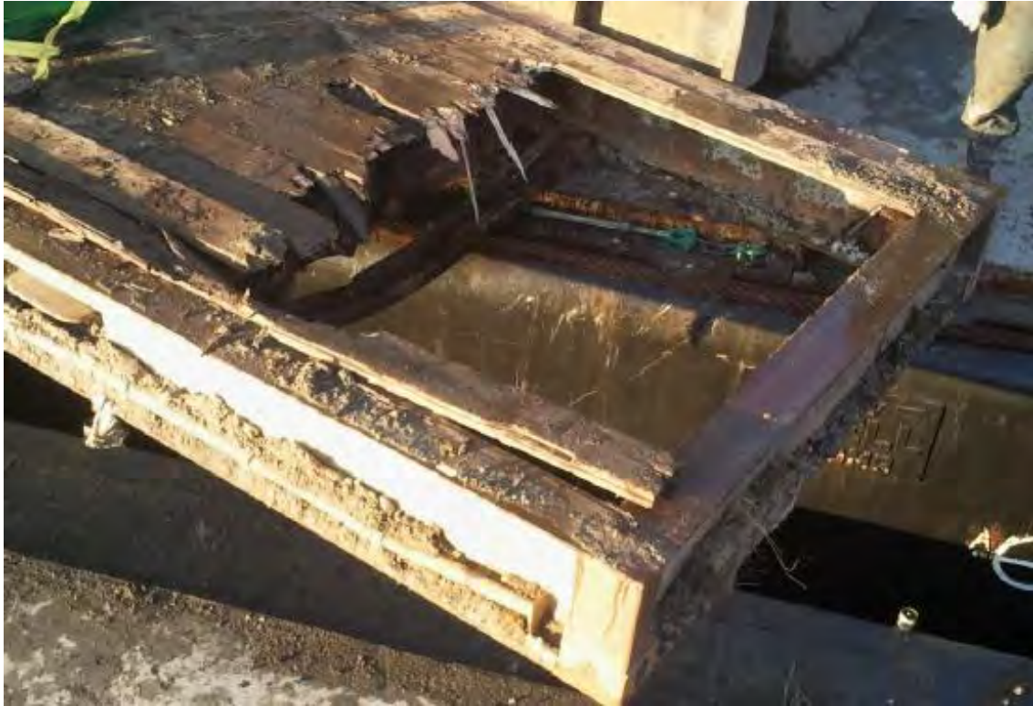
Photo 27: Failed wooden flat that resulted in a lost 5-CY super sack at Dillingham, Alaska, 2011
