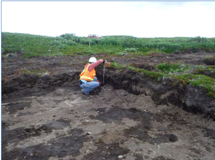
Photo No. 6 – 29 June 2016 Measuring walls within the tundra area to determine if wall sample collection needs to occur. View facing west.
