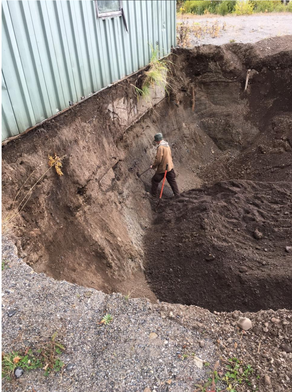
Photo 2: 6' auger depth (the auger extension had been added). About to collect samples BF-2 & BF-3.
