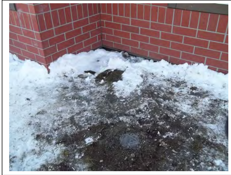
Photo 7: Looking southeast, a view of Monitoring Well B4MW, which was installed in Boring B4. (April 15, 2013)
