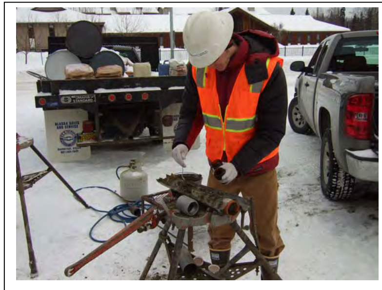
Photo 4: Shannon & Wilson personnel collected soil samples from the split spoon samplers using dedicated stainless steel spoons. This was Sample B3S4. (February 22, 2013)
