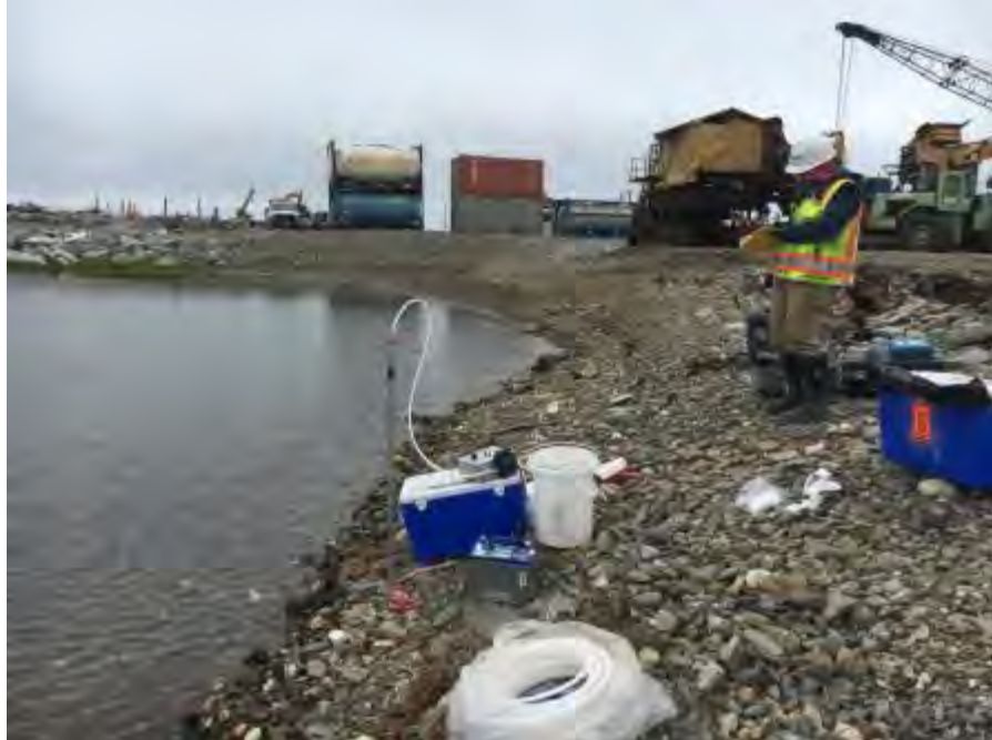
Photo No. 12 – 21 June 2016 Pore water sampling at location SP05. Pore water probes were installed with a slide hammer to 2 feet below ground surface during falling tide. Looking southwest.
