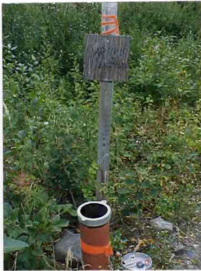
OUB: Poleline Road, Overcasing of Monitoring Well AP-4017.
