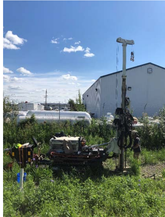
Photo 2: Direct push Geoprobe® 8040 track mounted drilling rig equipped with OIP technology.
