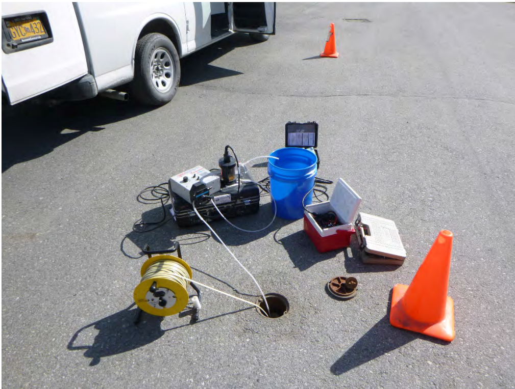
Photo 3: Monitoring Well MW-7 TS as it is being purged. Location is north of Transformer Shop. Photo on 6/10/2020.
