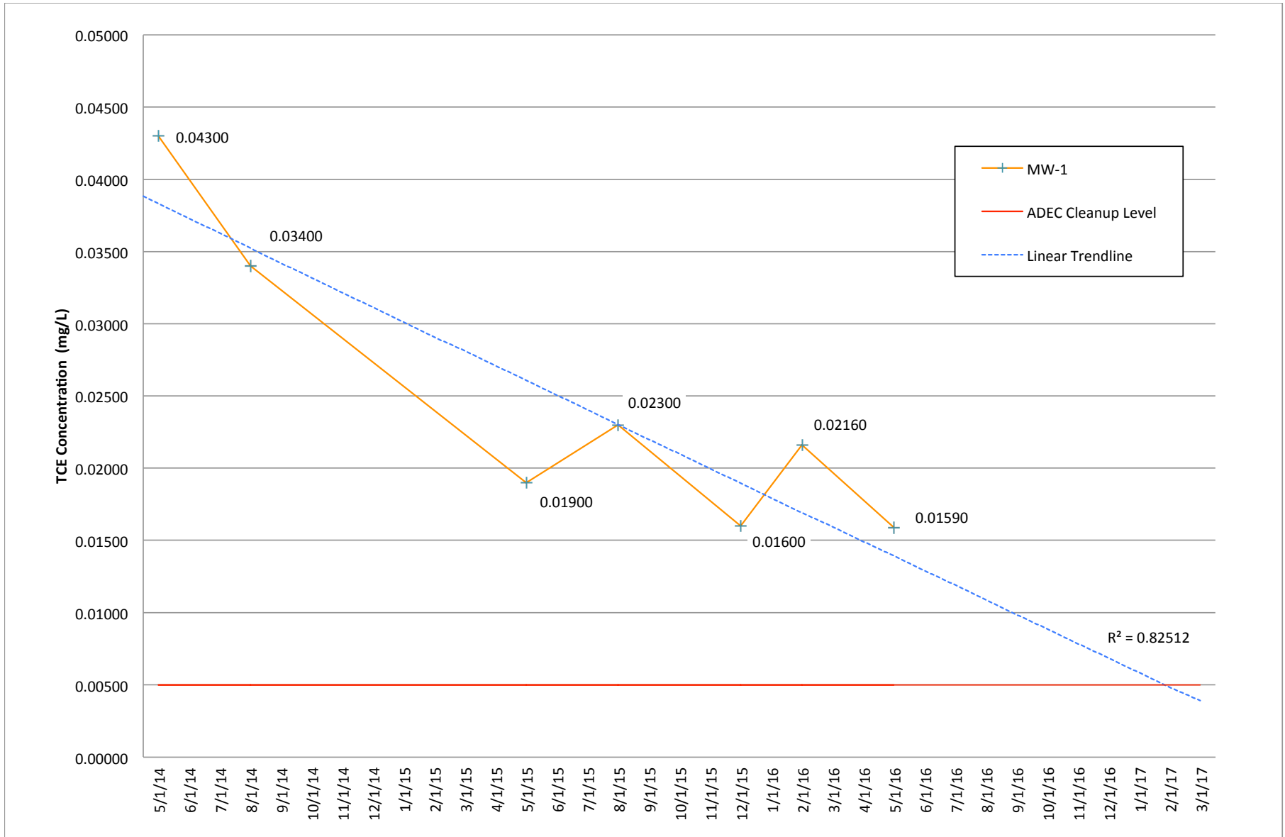
GRAPH 2: MW-1 TCE CONCENTRATION TREND Quarterly Groundwater Monitoring Report – May 2016 Nikiski Completions Facility Baker Hughes Oil Field Services, Inc. Nikiski, Alaska
