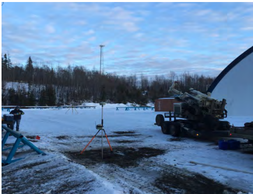
"MW-10" NAD83(2011) (EPOCH 2010.0000) 60° 43' 59.76521" N 151° 18' 05.37933" W Top of Case=130.45' Top of PVC Pipe=130.16' Ground Elevation=130.7' *February 2016 Value
