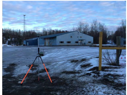
"MW-09" NAD83(2011) (EPOCH 2010.0000) 60° 43' 57.94219" N 151° 18' 07.56516" W Top of Case=129.30' Top of PVC Pipe=128.95' Ground Elevation=129.3' *February 2016 Value
