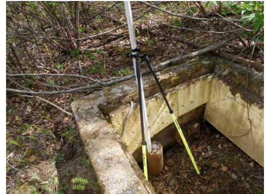
“McGhann Abandoned” NAD83(2011) (EPOCH 2010.0000) 60° 43' 53.02088" N 151° 18' 01.96405" W Top of Case=138.56' Ground Elevation=140.2' *May 2015 Surveyed Value
