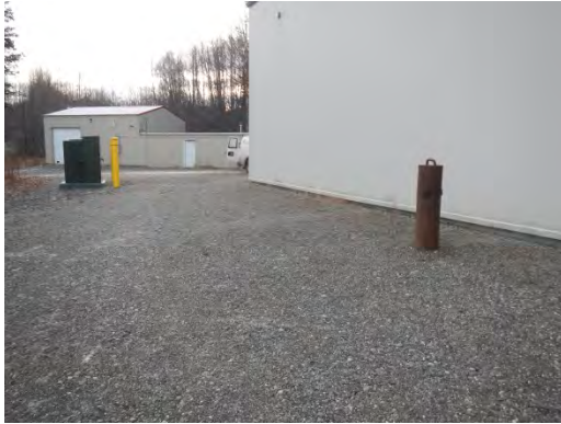
“McGhann Test Well” NAD83(2011) (EPOCH 2010.0000) 60° 43' 55.44320" N 151° 18' 06.41612" W Top of Case=138.65' Ground Elevation=135.6' *May 2015 Surveyed Value
