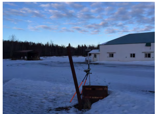
"Tuboscope Well" NAD83(2011) (EPOCH 2010.0000) 60° 43' 57.29254" N 151° 18' 22.17292" W Top of Case=130.10' Ground Elevation=129.8' *February 2016 Value
