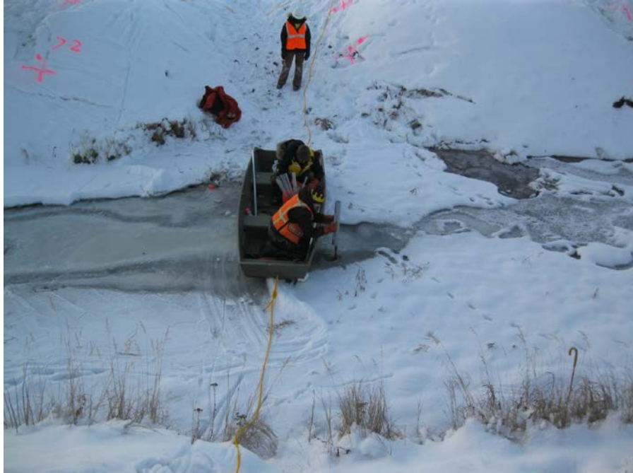
Photo No. 6 – 15 November 2012 Sub-sample acquisition using a fence post driver from boat at DU-7-2. View facing west.
