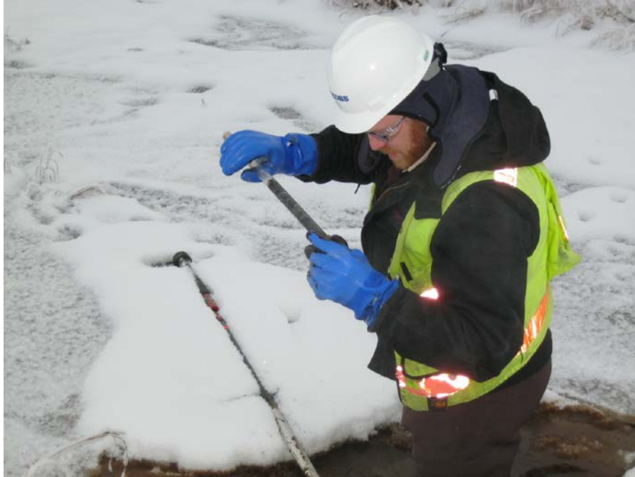
Photo No. 3 – 14 November 2012 Sample core retrieved using the single tube sampler. View facing northeast.
